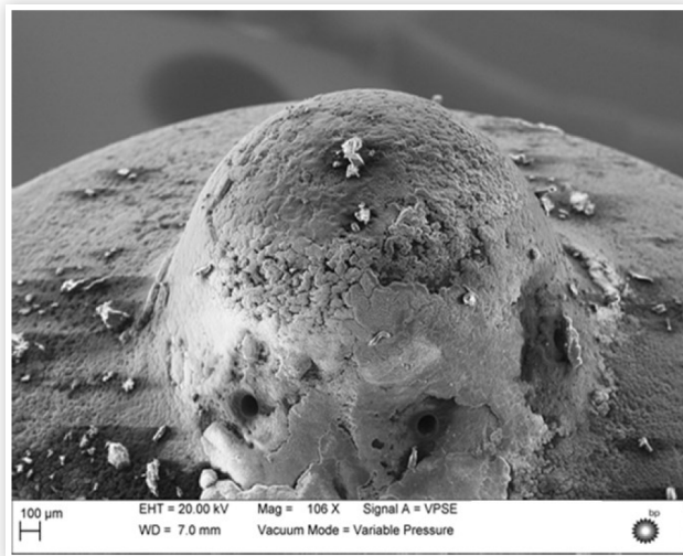
FIGURE 2 Deposits on the external surface of a diesel fuel injector.
